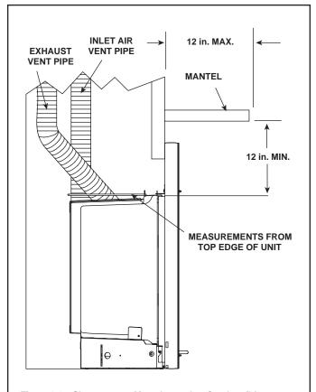
Figure 3.2 Clearances to Mantels or other Combustibles above Appliance
